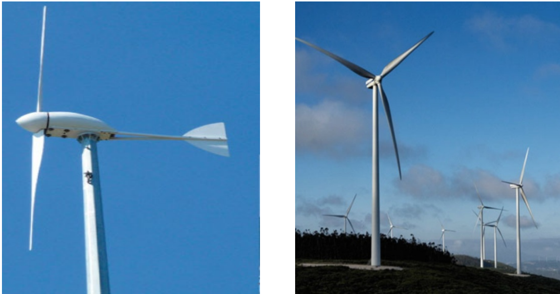
Figure 34:- Horizontal Axis Wind Turbines
