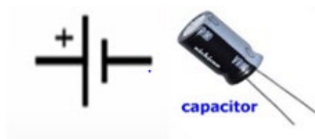
Figure 11: Electrolytic Capacitor and its Symbol
