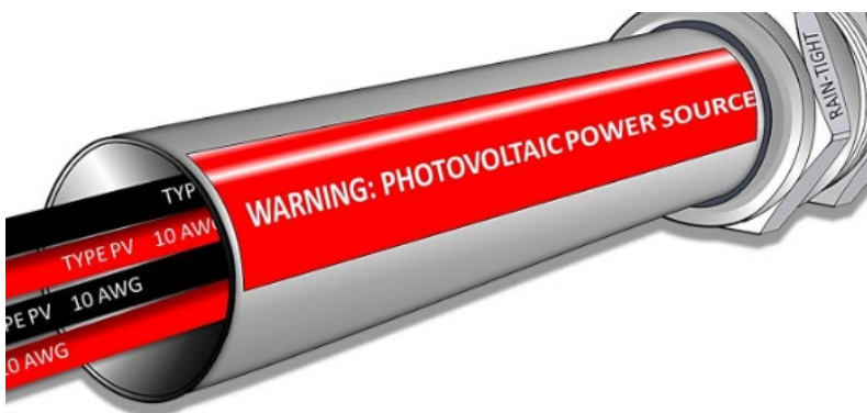
Figure 42: PV cable in conduit ( https://www.jadelearning.com/ )
