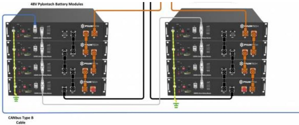
Figure 80: Battery Connections (Pylontech)
